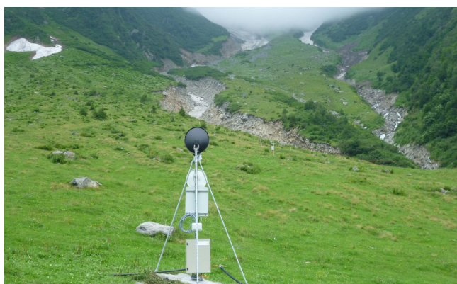
Figure 2: Radar measurements are used to detect movements in the rupture zone of the debris flow.
