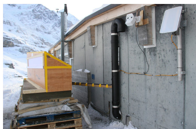
Figure 3: The interferometric radar is well protected by a wooden case. Next to it, a camera and the avalanche radar also look at the glacier.
